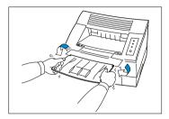
2 Slide the lower part of the paper feed tray into the printer.
